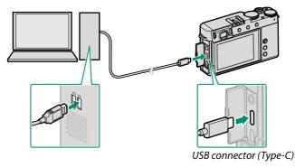
① The USB cable must be no more than 1.5 m (4.9 ft.) long and be suitable for data transfer.
